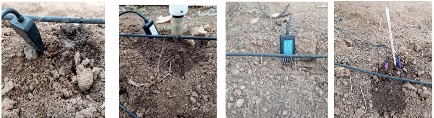
Figure 23. Soil sensor buried into the ground
