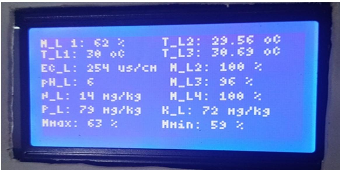
Figure 25. Real-time parameters of the soil
