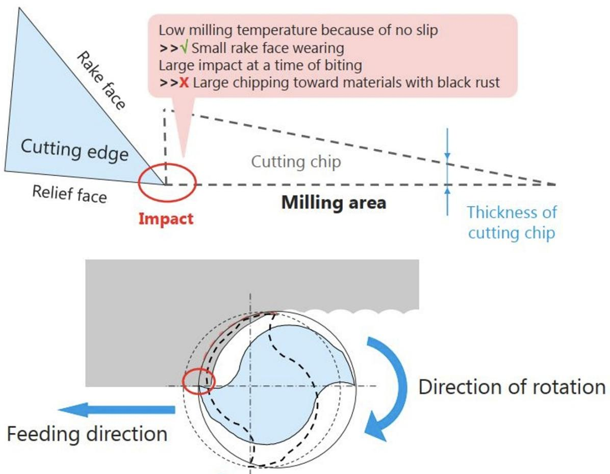
Figure 2. Down milling Physics in milling [13]
