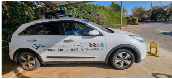
Figure 1. Left image: The lab vehicle equipped with a multi-sensor kit, including the InnovizOne LiDAR mounted at the front of the roof. Right image: A close-up of the InnovizOne LiDAR mounted on the vehicle's roof
