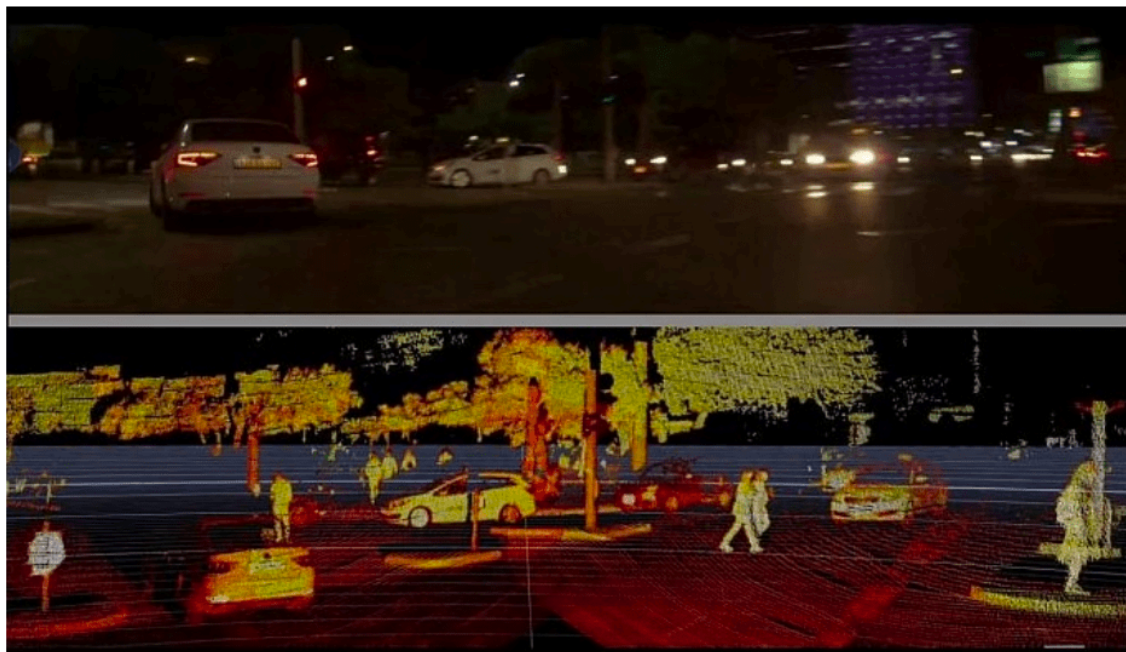
Figure 2. The image shows a traditional camera view at night, where pedestrians are difficult to spot due to poor lighting. The bottom image, generated using Innoviz LiDAR data, reveals a much clearer and detailed scene, detecting pedestrians and vehicles even in complete darkness. This demonstrates how LiDAR technology excels in low-light environments, offering critical advantages for autonomous systems. [7]
