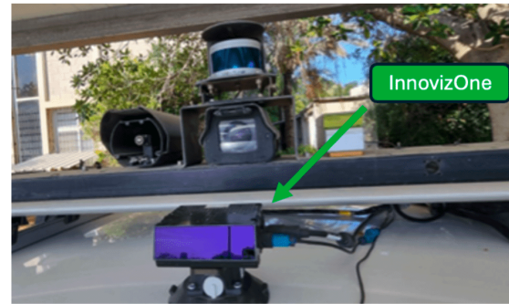
Figure 1. Left image: The lab vehicle equipped with a multi-sensor kit, including the InnovizOne LiDAR mounted at the front of the roof. Right image: A close-up of the InnovizOne LiDAR mounted on the vehicle's roof
