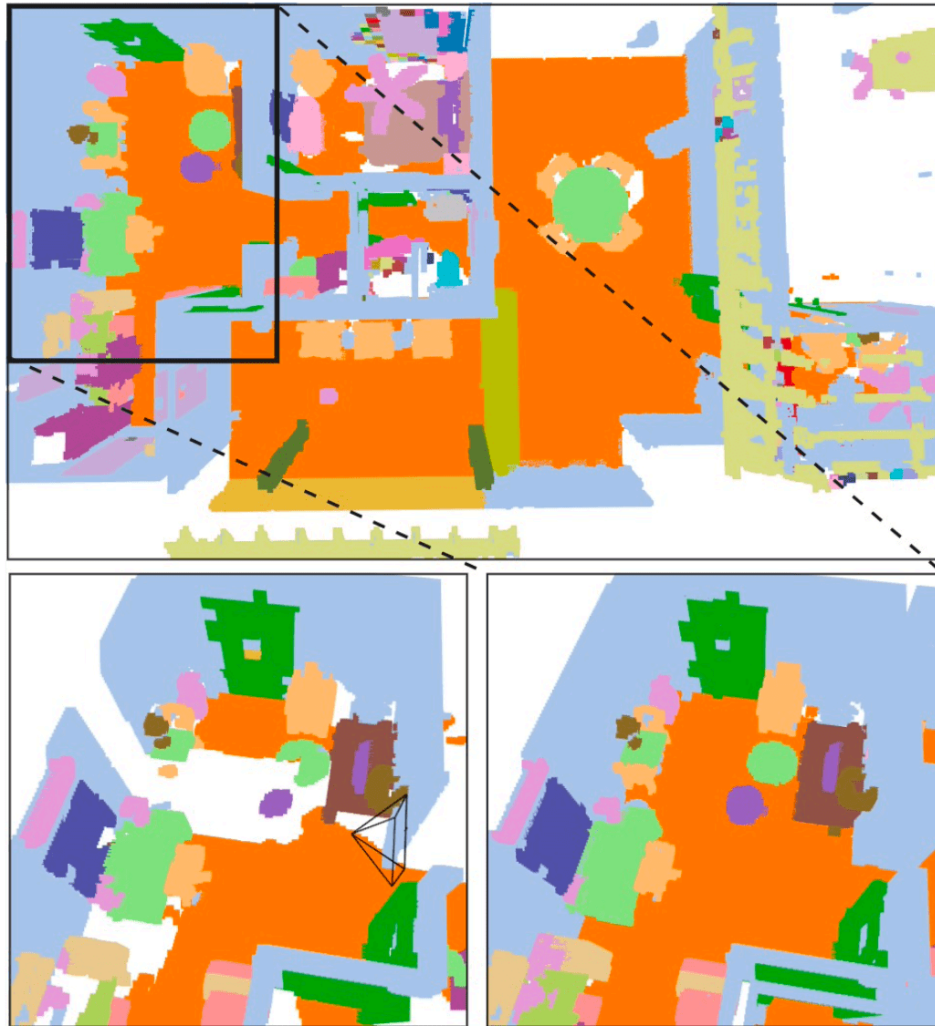
Figure 5. Language map incrementally created with our adaptive optimization. Bottom Left: A region mapped in the beginning. Bottom Right: The same region after the mapping is completed. All initially mapped objects remain unchanged.
