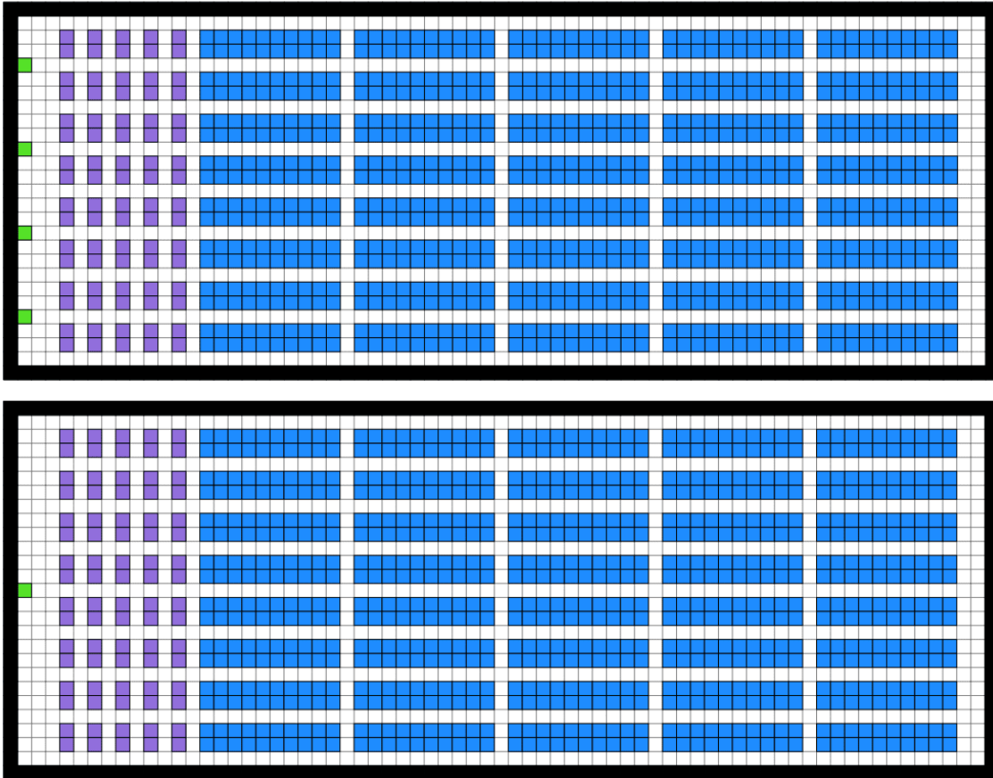
Figure 1. Warehouse maps: (1) Blue grids represent shelves S . (2) Purple grids represent caches C . (3) Green grids represent unloading ports U . The upper map has multiple ports, while a single port is in the bottom one. In the multi-port map, each unloading port is associated with its own independent cache area, task queue, and set of agents. The cache areas are located near the unloading ports, within a range of \pm 2 rows. In contrast, the single-port map allows the port to utilize all available agents and caches. Given that the number of cache grids can influence the cache hit rate, we tested different configurations by varying the number of cache grids from 80 to 16. This was achieved by progressively removing cache grids column by column from right to left.
