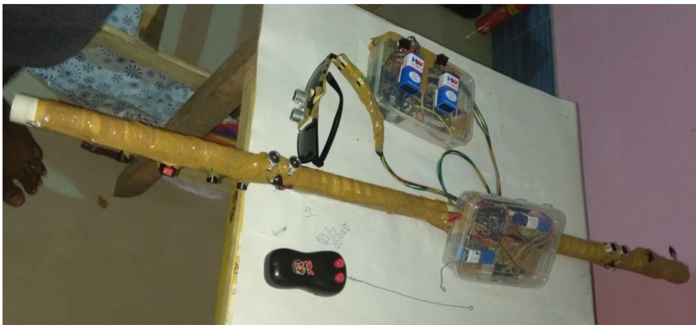
Figure 6. Prototype of the smart stick for blind people.
