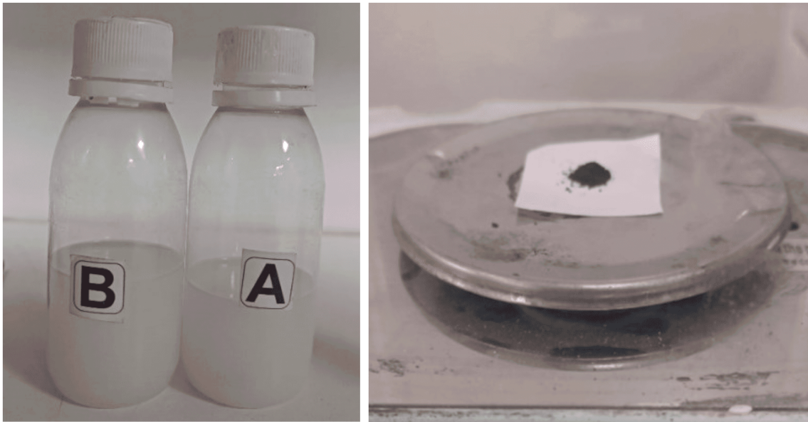
Fig. 3.4. Commercial Ecoflex Part A and Part B and Measured Graphene nano-powder
