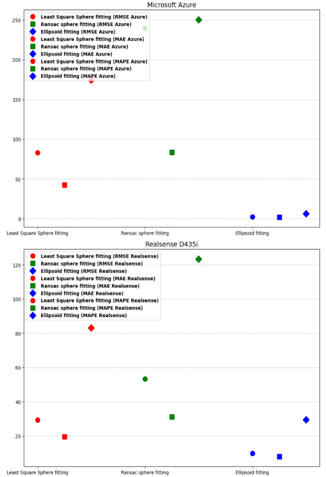
Figure 11: RMSE, MAE, MAPE, and R-squared distribution achieved using the 3 shape fitting techniques on the images collected using Microsoft Azure camera and IntelRealsense D435i camera.
