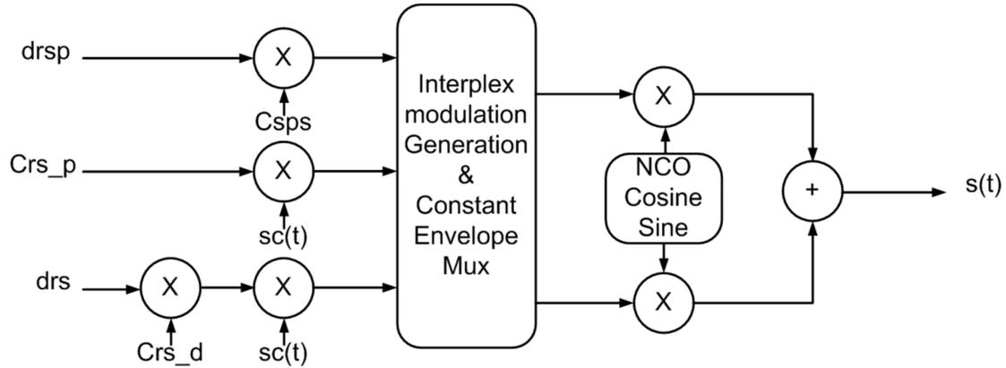
Figure 2. Block schematic for composite signal generation
