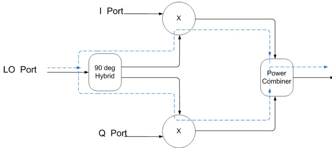
Figure 3. Leakage path in Mixer
