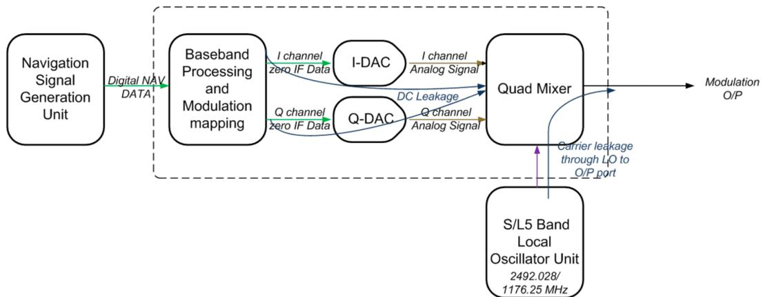
Figure 4. Leakage path in modulator
