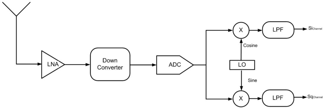
Figure 7. Block Diagram of GNSS Receiver
