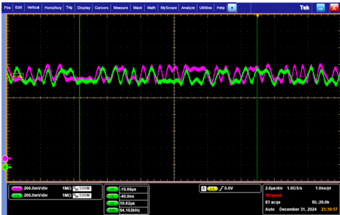
Figure 6. Time domain waveform of I and Q Channel with IQ offset
